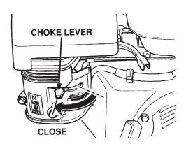
Figure 22. Choke Lever (Closed Position)
